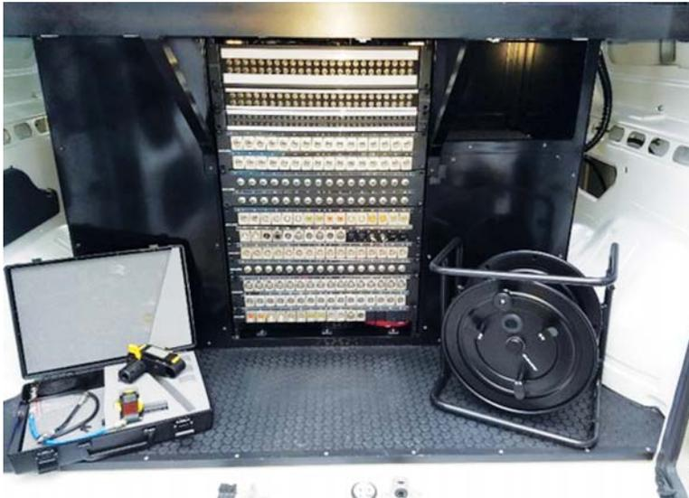
Most 12G-SDI solutions are installed in the rear part of the car.
