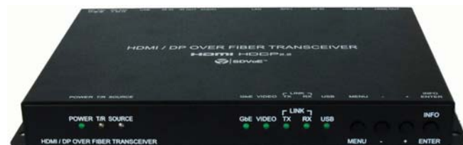
SFP+ version of SZ-TR6 converter(Tx/Rx)
